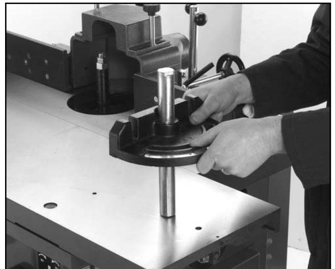
Figure 20. Installing the miter gauge.
